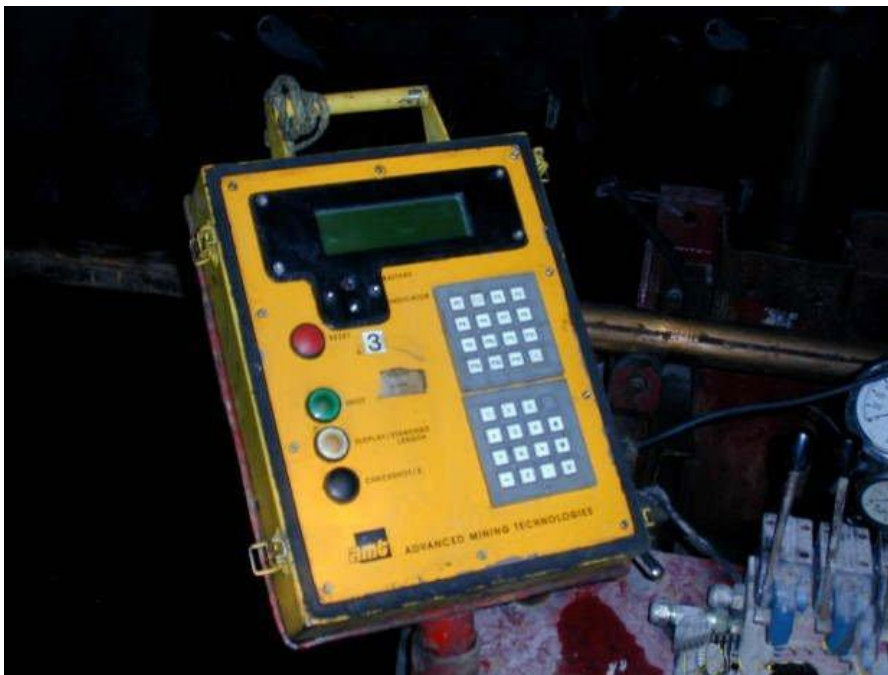
Figure 2 DDM MECCA uphole monitor box calculates and displays high resolution survey data.
