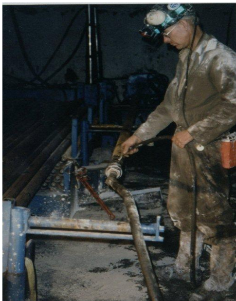
Figure 3 Surveys take less than 5 seconds after connecting MECCA to uphole monitor box with signal cable.
